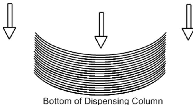
A wide opening at the top of each column allows you to enter stacks of tickets. Grasp a manageable stack of tickets. Slide the stack down the chute. Continue to load tickets until the column is full. **All tickets in one column must be of the same value.**
