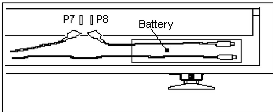
Plug in the two connectors as illustrated. The display on the console will now read ALARM ACTIVATED ENTER PIN NUMBER.
