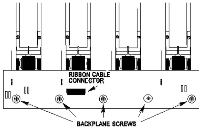
4. Disconnect the 14 Conductor Ribbon Cable located on the back plane and remove the five Philips screws from the backplane.
