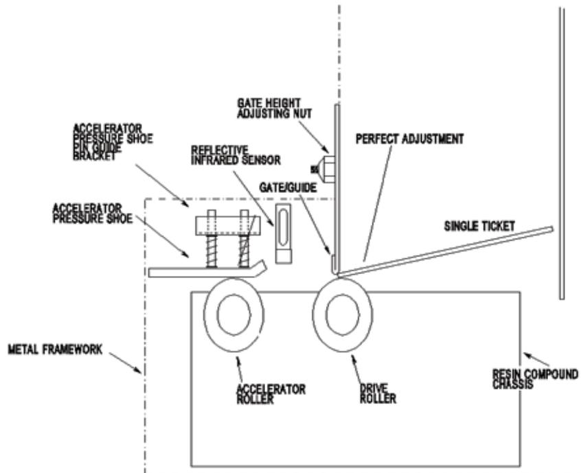
2. Adjust upwards for thicker tickets. Adjust downwards for thinner tickets.
